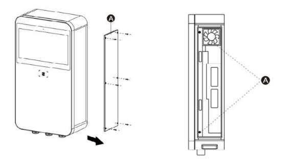
3. Press the button (A - bottom) and slide the card tray to the right to remove it. Place the SIM card into the card tray. Ensure the car is inserted correctly. Reinstall the card tray
