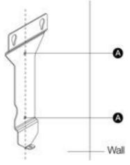
4. For rear entry wiring, mark the cable exit where the AC input cable will come out from the wall. Ensure that the cable exit matches the wall dock notch according to the diagram below.
