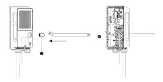
4. Remove the lower-left cable gland and install the bottom entry power conduit plug (E) to the charger.
