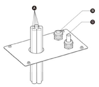
Figure 5-9 Guiding the Cables through the Cable Gland Plate
