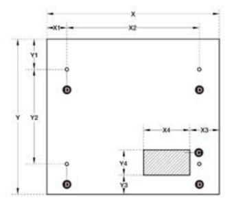
Figure 4-4 Foundation Diagram
