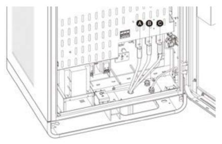
Figure 5-13 Connecting the AC Input Wires (1)
