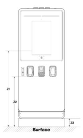
Figure 9-1 Operable Element Specifications
