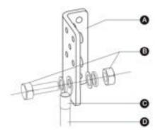
Figure 5-11 Connecting the PE Wire (2)
