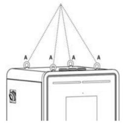
Figure 5-2 Hoisting the Cabinet
