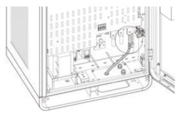
Figure 5-10 Connecting the PE Wire (1)
