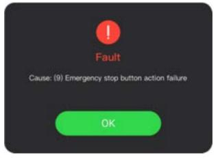
Figure 6-1 Fault Message Screen
