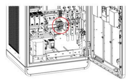
Figure 6-7 Measuring the AC Voltage
