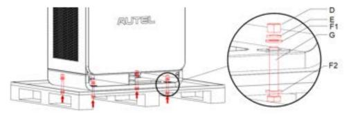
Figure 5-7 Removing the Cabinet from the Pallet
