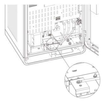
Figure 5-12 Grounding the Enclosure
