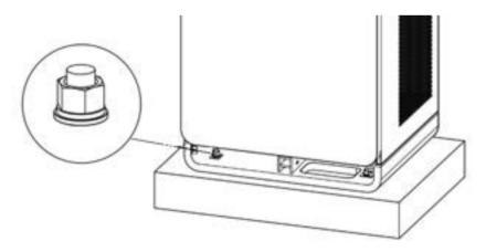
Figure 5-8 Tightening the Bolts
