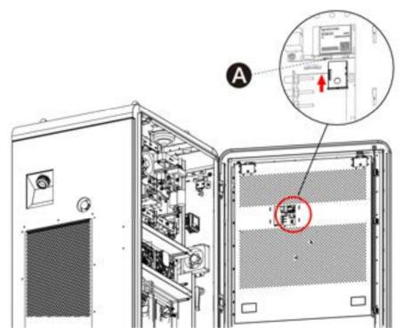
Figure 5-16 Installing the SIM Card
