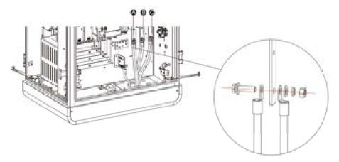
Figure 5-14 Connecting the AC Input Wires (2)
