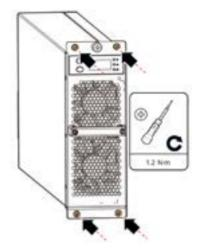
Figure 5-20 Tightening the Screws
