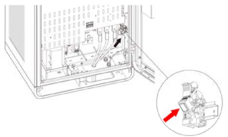
Figure 5-15 Connecting the Ethernet Cable
