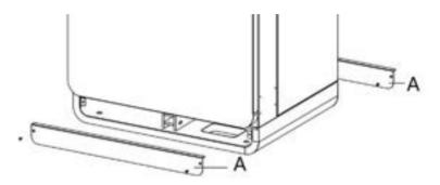
Figure 5-4 Removing the Base Covers
