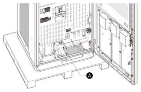
Figure 5-6 Loosening the Fasteners
