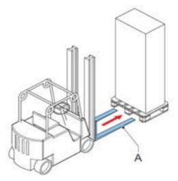
Figure 5-3 Transporting the Cabinet by Forklift
