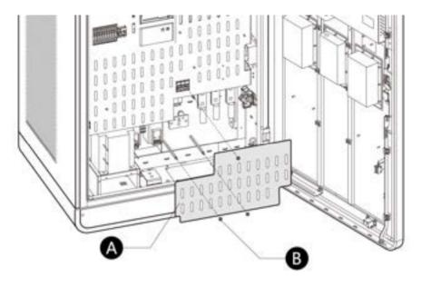
Figure 5-5 Removing the Galvanic Isolation Board
