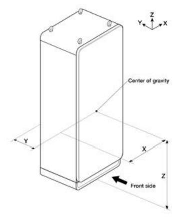
Figure 5-1 Center of Gravity
