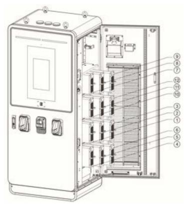
Figure 5-19 Installing the Charging Module (for MaxiCharger DC 240) Table 5-2 Charging Module Installation Specifications
